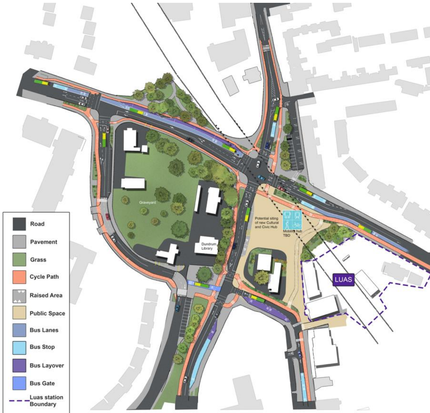
Figure 6.5 ABTA Recommendations for Taney Cross illustrating an indicative junction layout
