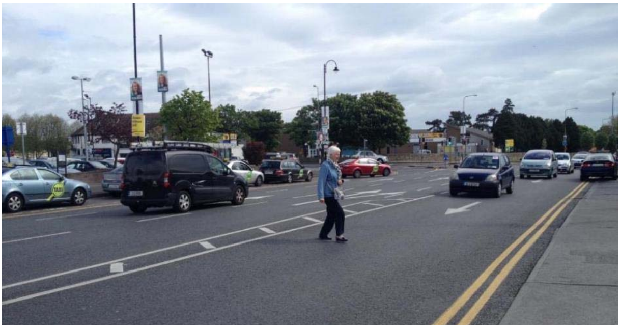
Figure 2.4: Pedestrian crossings do not match desire lines, encouraging pedestrians to cross wide carriageway with no crossing facilities
