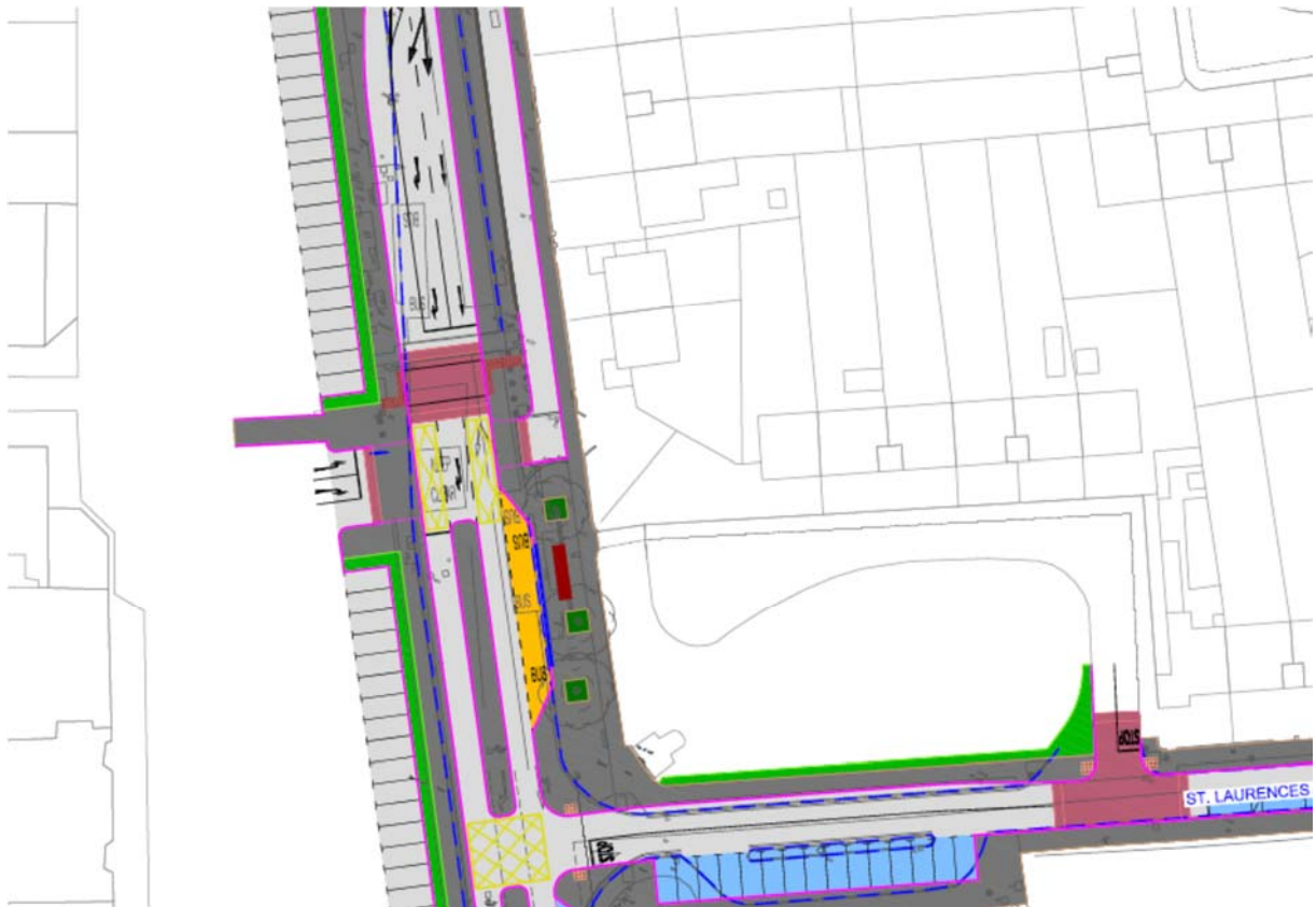
Figure 5.8: Proposed Junction Layout
