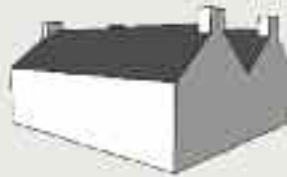
Double 'A' roof with central valley
