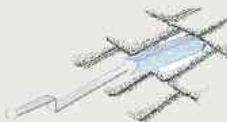
Here, a partially folded metal piece is slid under the upper slate as part of the bib repair. The metal is partially folded to allow the metal to sit above the nail head. The metal used should preferably be a painted aluminium or copper but should be matt in texture
