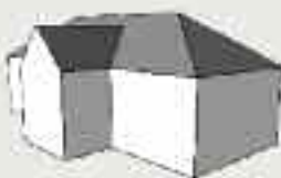
Hipped roof with gabled entrance
