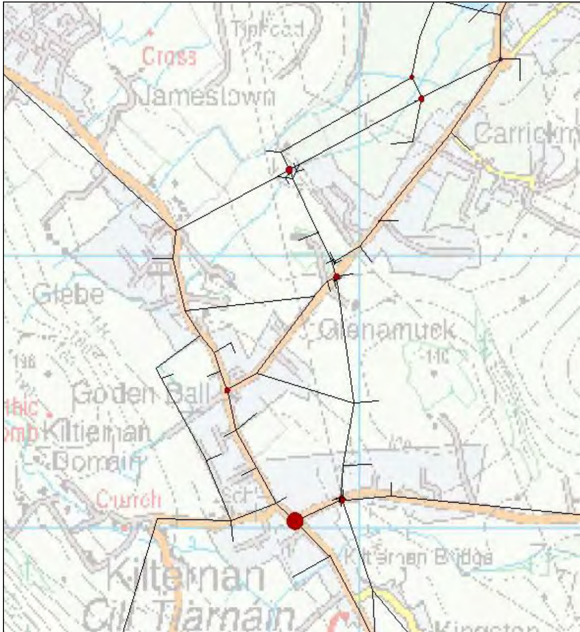
Figure 5.35 Junction Delays and Blocking Back on Option 4 Network
