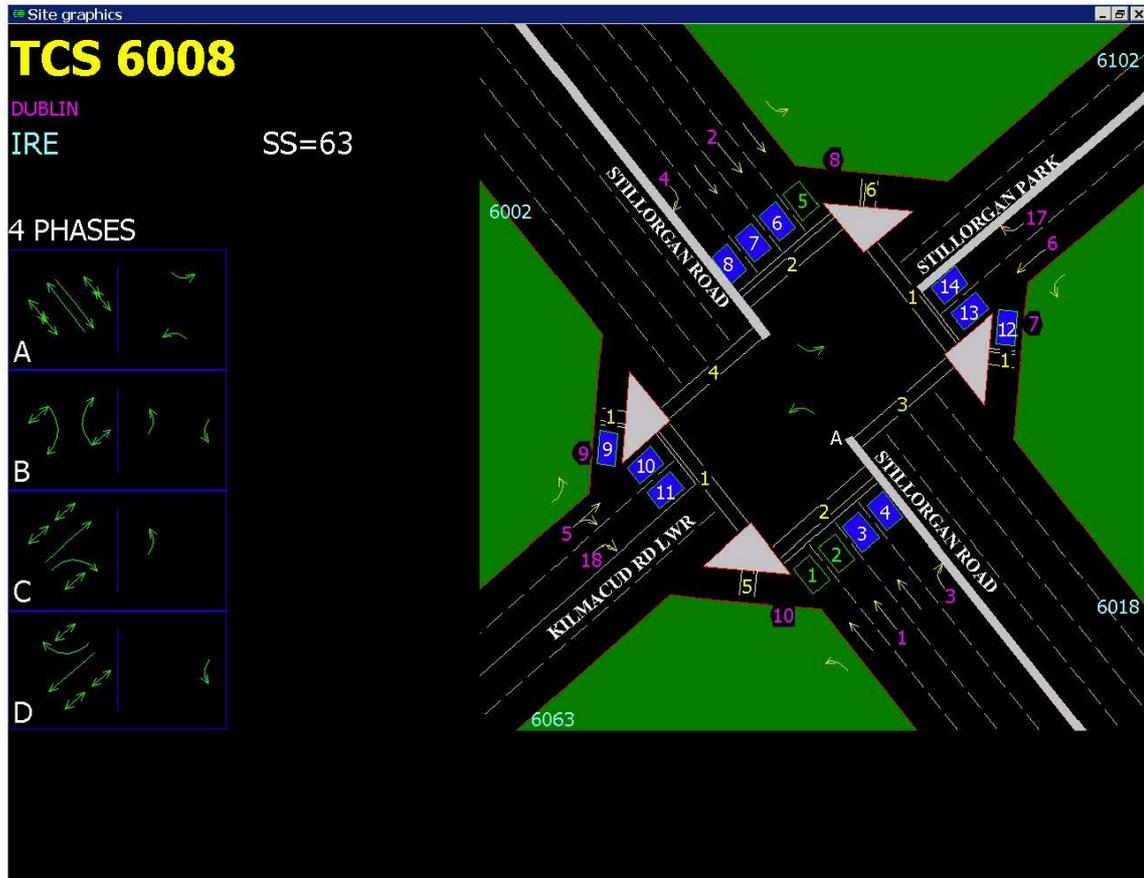
Figure 4.5 Existing Traffic Signal Plan
