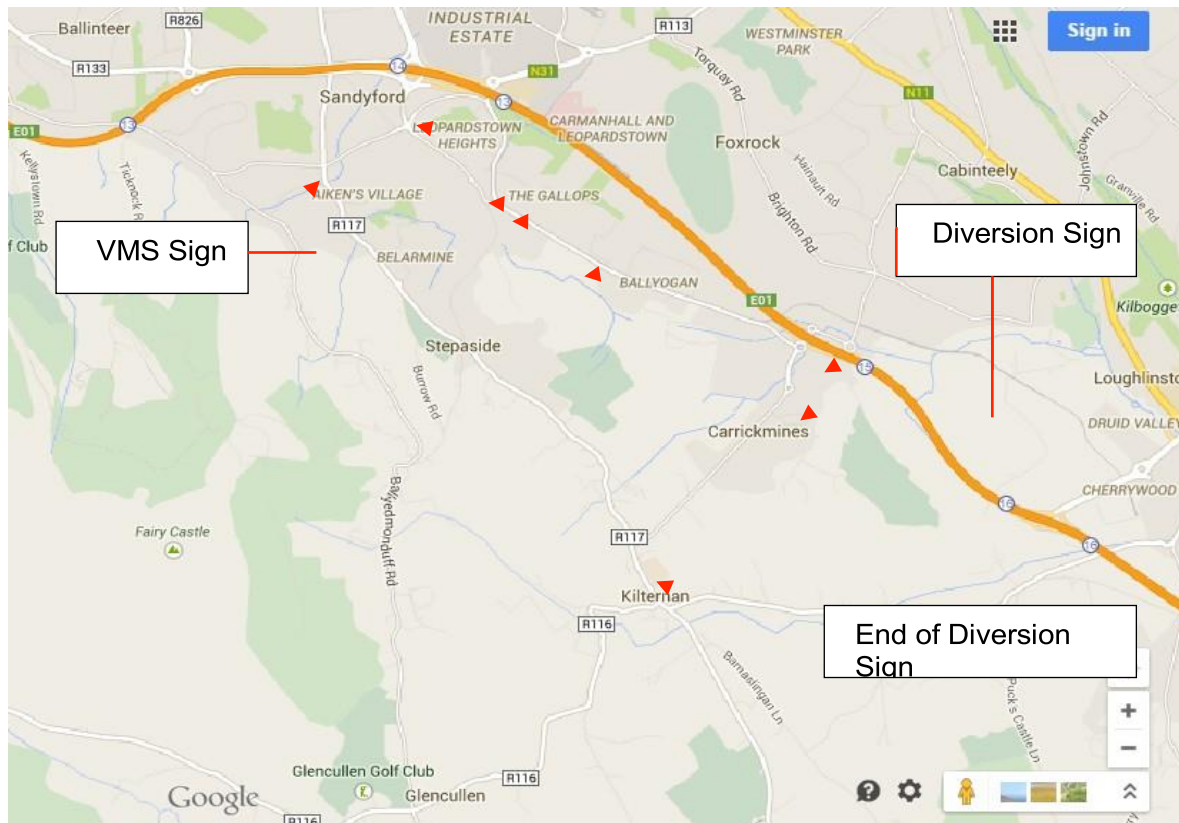
Diversion No. 3 -- Location of Diversion Signs
