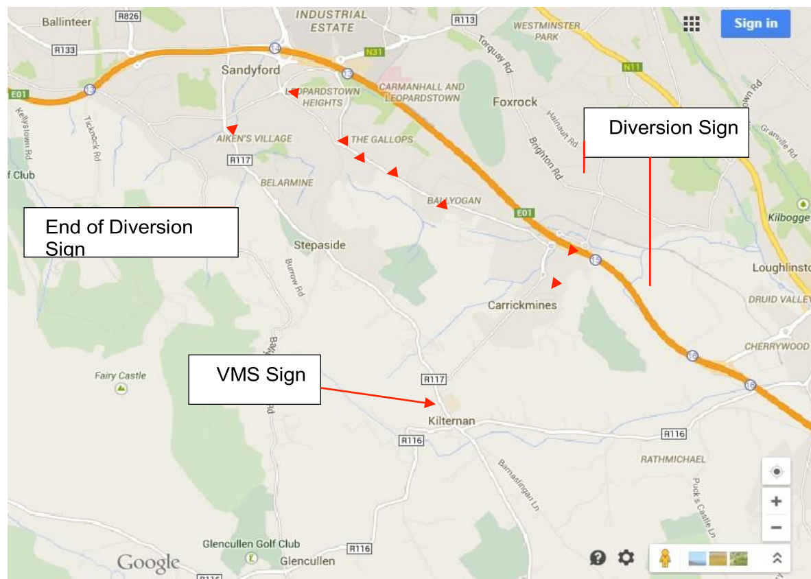
Diversion No. 1 -- Location of Diversion Signs
