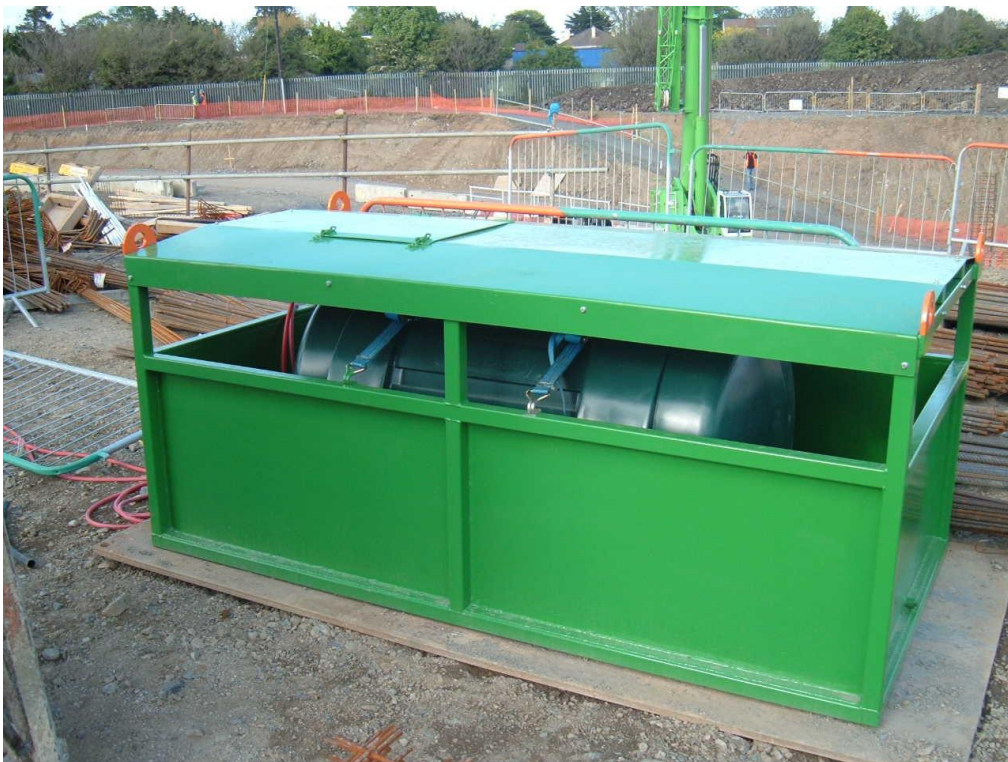
Photo 1: Typical bunded and covered storage tank as available from the Plant Department
