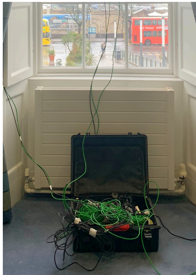
Thermal transmittance and surface temperature monitoring sensors attached to the single glazing and wainscot panels behind the radiators.
