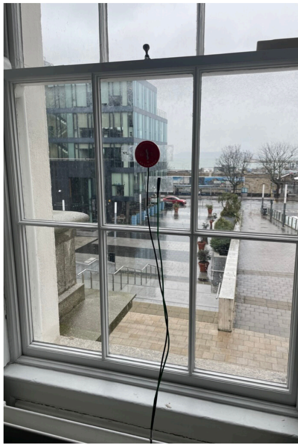
Thermal transmittance and surface temperature monitoring sensors attached to the single glazing and wainscot panels behind the radiators.
