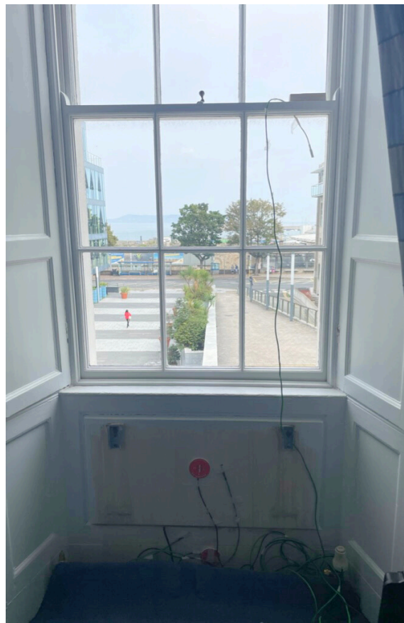
Thermal transmittance and surface temperature monitoring sensors attached to the single glazing and wainscot panels behind the radiators.
