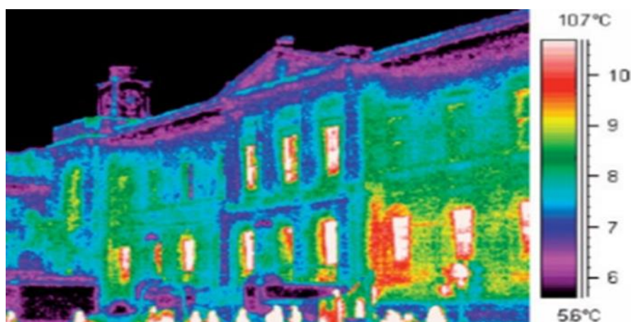
Figure 1 A graphic illustration of heat loss from a building in Edinburgh: most of the windows are single-glazed and are emitting more heat than the thermal imaging camera can record (the white areas); six windows on the top floor (the green areas) have secondary glazing and are cool.
