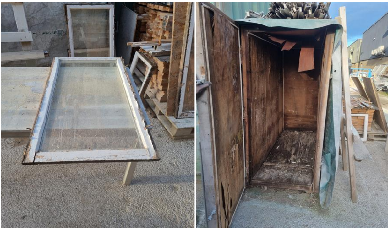
Figure 2 Window for refurbishment & steaming box
