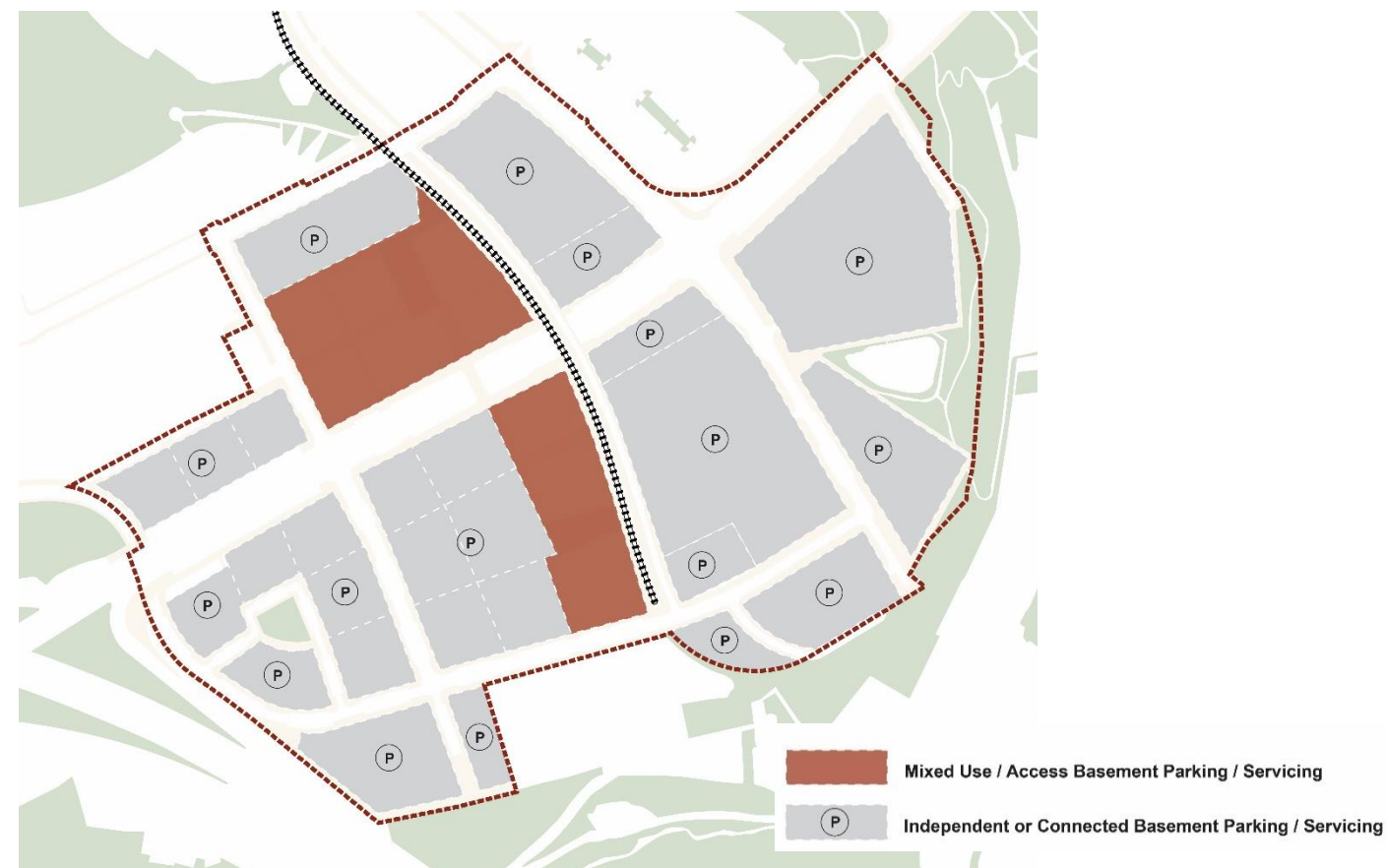
Figure 20. Overall concept for land use below ground/basement
