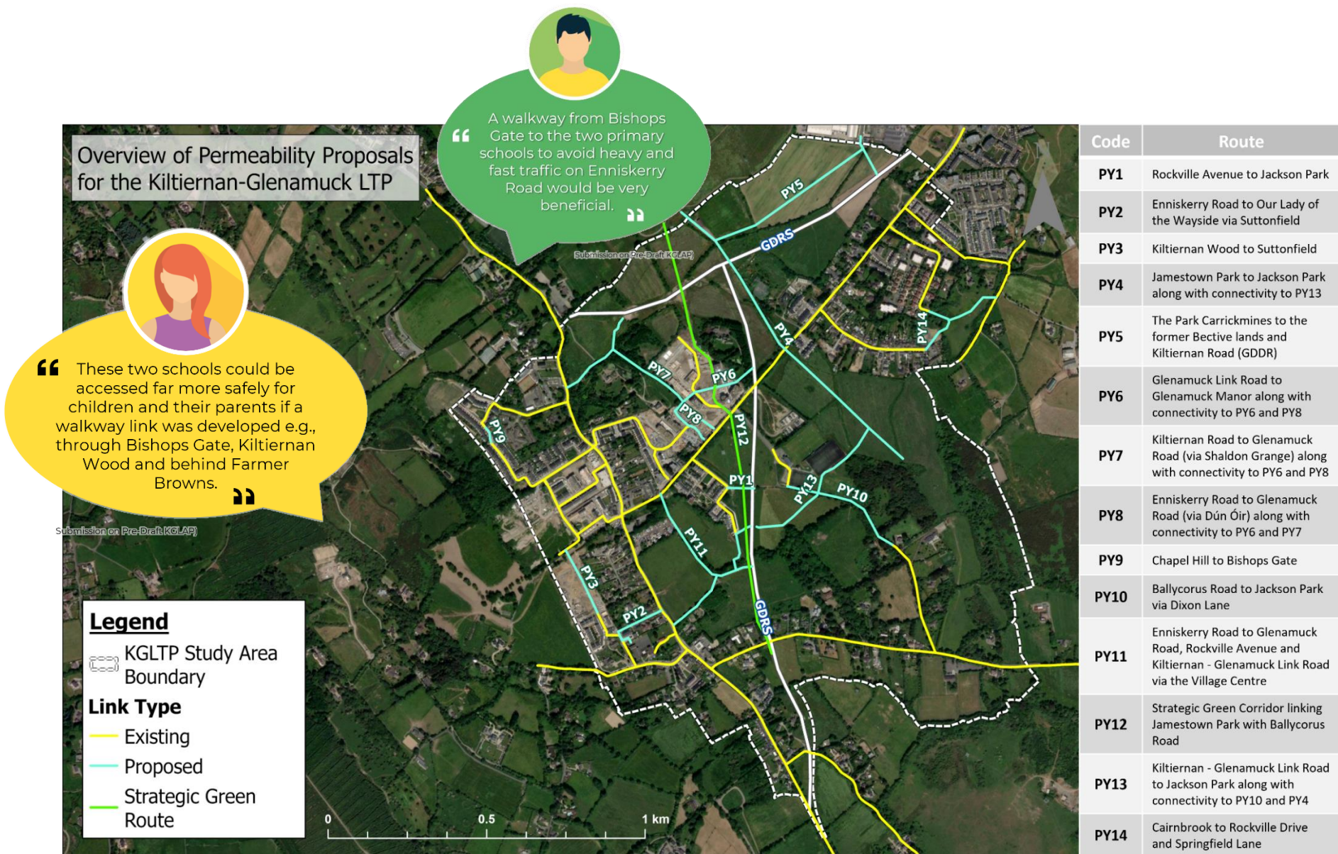
Figure 11-4: Map of proposed permeability links for the Kiltiernan-Glenamuck area, alongside existing links. Source: DBFL.
