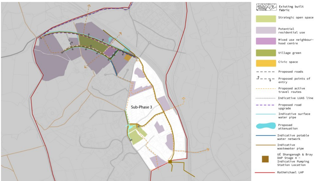
Figure 3-17: Rathmichael Phase B Sub-Phase 3 Infrastructure (For context, please see the overall Rathmichael Proposed Infrastructure Phasing Map in Appendix D)
