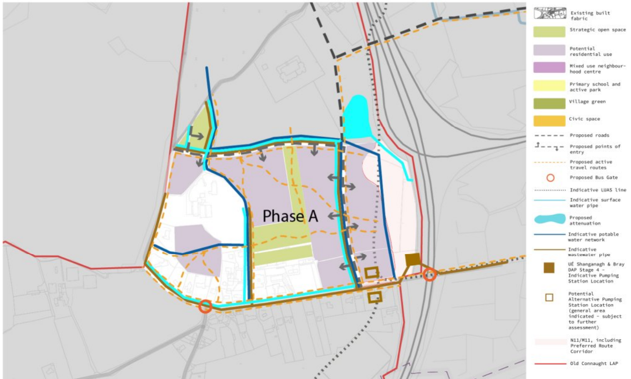
Figure 3-3: Old Connaught Phase A Infrastructure (For context, please see the overall Old Connaught Proposed Infrastructure Phasing Map in Appendix D)
