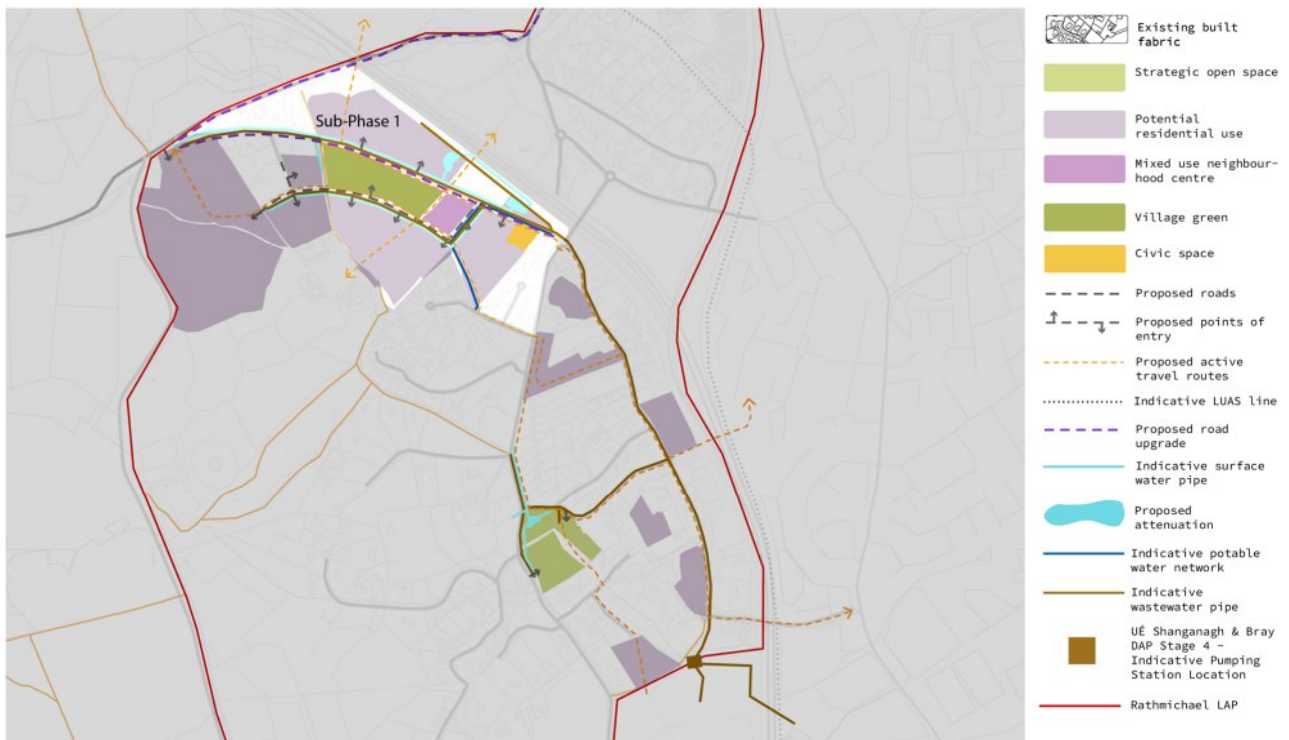
Figure 3-15: Rathmichael Phase B Sub-Phase 1 Infrastructure (For context, please see the overall Rathmichael Proposed Infrastructure Phasing Map in Appendix D)
